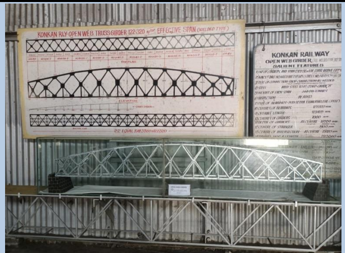
Kokan Railway Open Web Girder (122.32 m Span)
